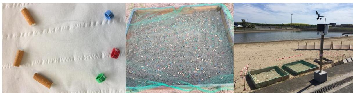
Figure 4: Tagged CB (left), CB deposited on Cedre artificial beach (middle) and view of the beach with CB weathering facilities and the weather station (right) (©Cedre).
