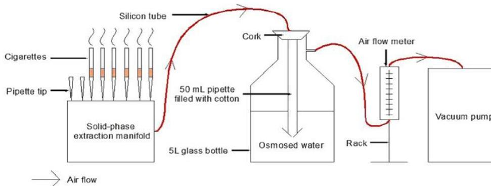
Figure 2: Equipment used to produce artificially-smoked CBs (©Cedre).
