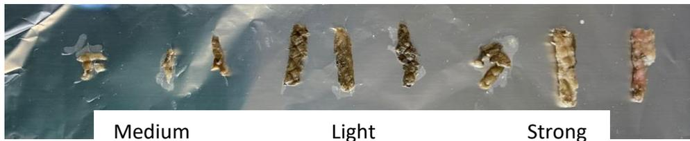
Figure 29: The three types of CB after 9 months of ageing on the Brest harbor seafloor.
