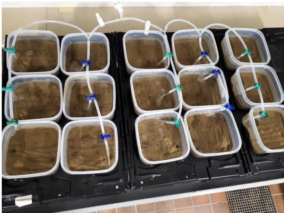
Figure 11: *Arenicola* test set up for cigarette butt testing (©Cefas).
