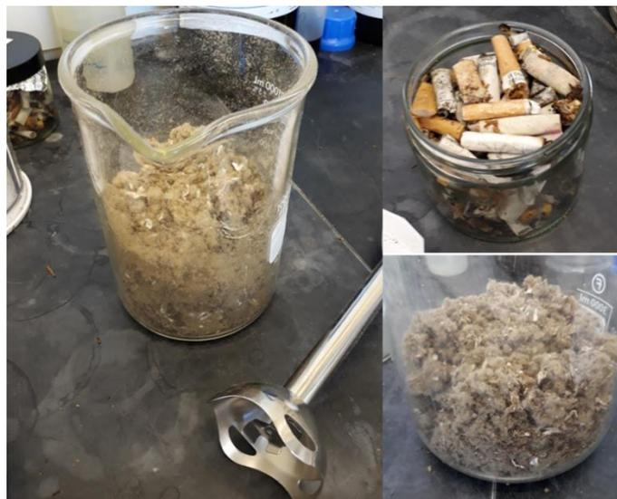
Figure 10: Homogenised CBs and stainless steel chopping/blending equipment (©Cefas).
