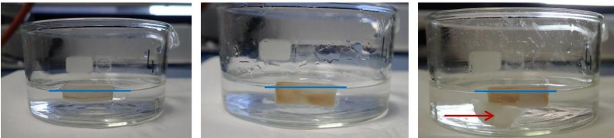
Figure 24: Behaviour of a medium-strength CB at 150 rpm at (a) 10 seconds, (b) 24 hours and (c) 20 minutes with the white paper starting to deteriorate (red arrow). The blue line represents the surface of the water
