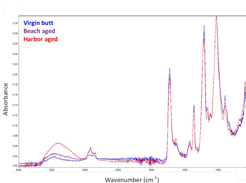
Figure 14: Absorbance spectrum for a fresh medium strength CB (blue) compared to the spectrum shown by the medium strength CB aged on the beach for 85 days (purple) or aged in the harbour for 70 days (red) (©IEO). (See also Santos-Echeandía et al., 2021).
