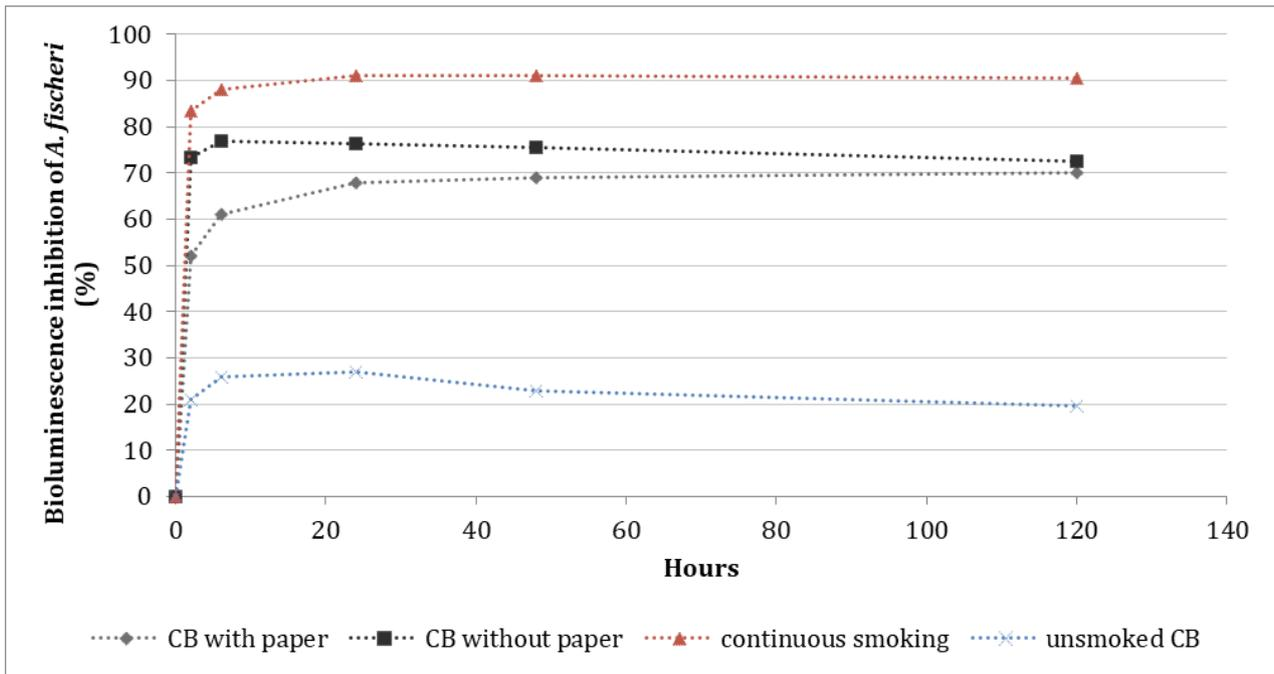
Figure 39: Mean bioluminescence inhibition (%) of *A. fischeri* by medium-strength CB leachate at a concentration of 10 CBs/L as a function of leaching time (hours) and type of CB used: with papers (n=1), without papers (n=2), continuous smoking (n=2), and unsmoked filters (n=2).
