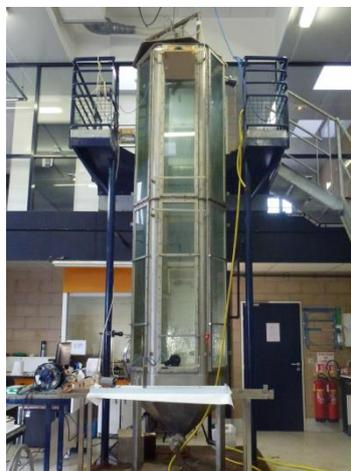
Figure 3: Cedre experimental column filled with natural filtered seawater (5-meter high) (©Cedre).
