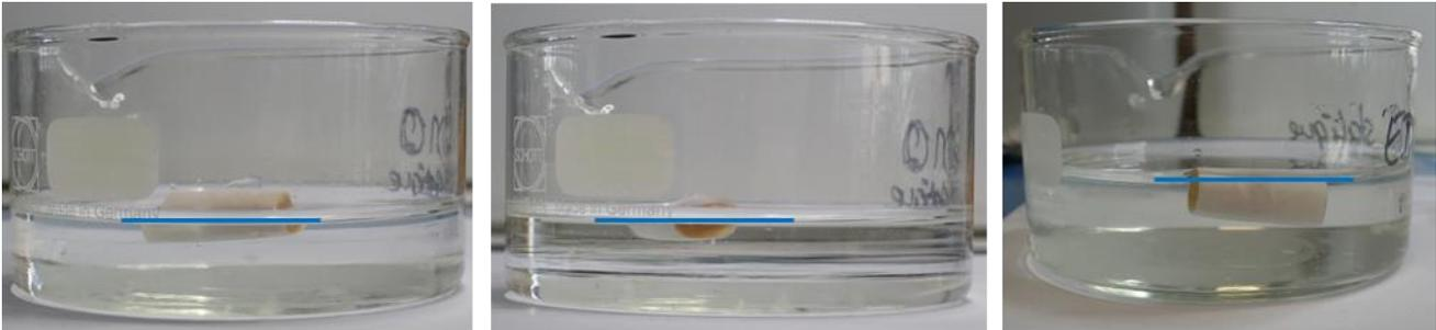
Figure 20: Behaviour of a medium-strength CB in seawater in static condition at (a) 20 seconds, (b) 40 seconds and (c) 24 hours. The blue line represents the surface of the water.
