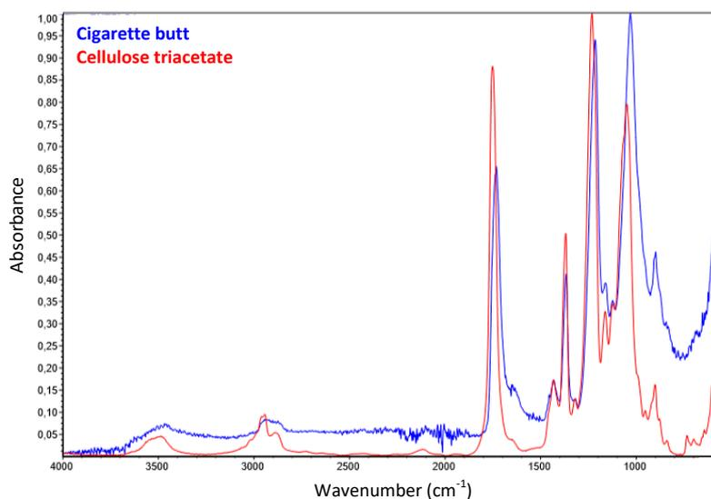
Figure 13: Typical absorbance spectrum for cellulose triacetate (red) compared to the spectrum shown by one of the CB used in the present study (©IEO). (See also Santos-Echeandía et al., 2021).
