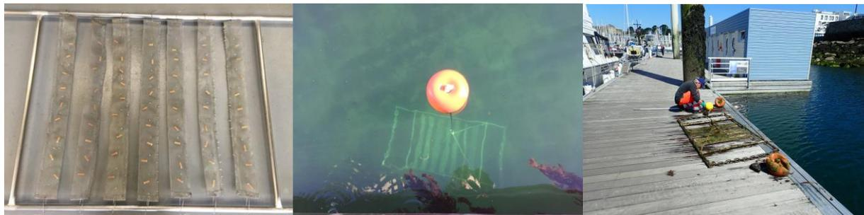
Figure 5: Photos of the deployment of CBs in stainless steel cages to monitor degradation processes over 1 year in Brest “Marina du Château” and in Cedre facilities (©Cedre)
