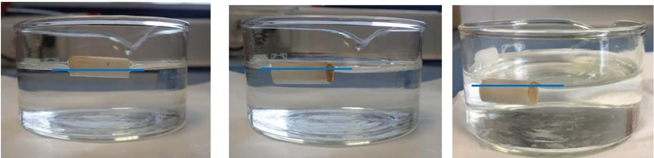
Figure 23: Behaviour of a medium-strength CB in seawater at 60 rpm at (a) 10 seconds, (b) 20 seconds and (c) 24 hours. The blue line represents the surface of the water.
