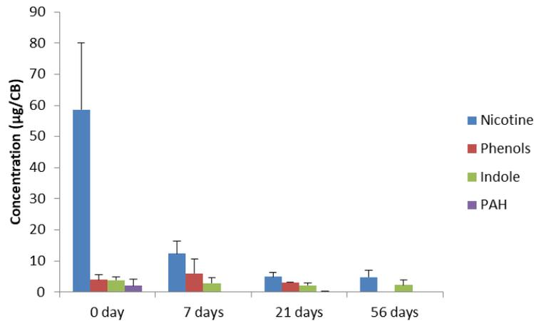
Figure 34: Concentrations of organic compounds in medium-strength artificial butts ( $\mu\text{g}/\text{CB}$ ) during 56 days of deployment on Cedre's artificial beach ( $n=3$ , means  $\pm$  SD).
