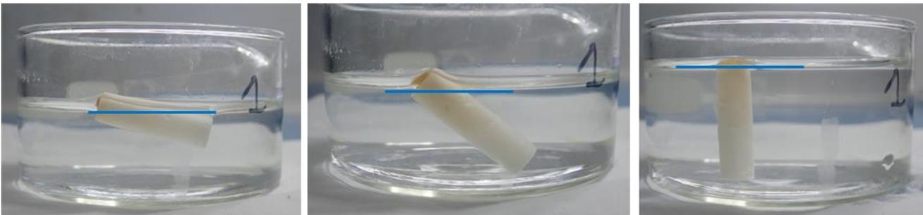
Figure 21: Behaviour of a light CB in seawater in static condition at (a) 20 seconds, (b) 40 seconds and (c) 24 hours. The blue line represents the surface of the water.
