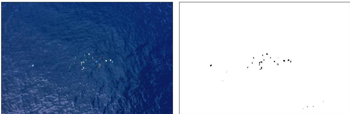
**Figure 4:** Pixel base detection of floating debris using colour difference to generate binary image (right) and estimate the proportion of floating debris pixels (%).
