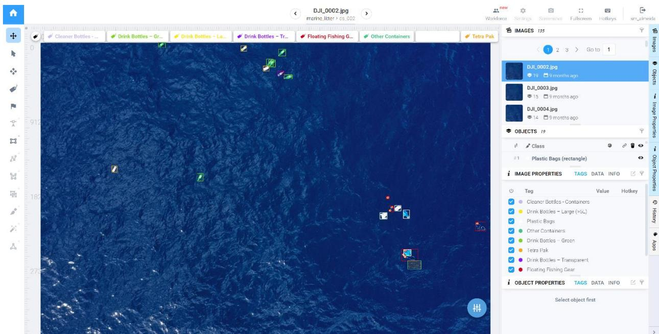
**Figure 5:** Example of Supervisely interface. Used to create the initial annotation automated detection and classification using deep learning.
