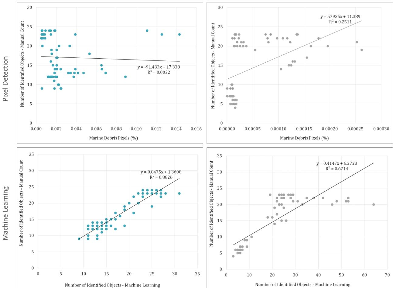
**Figure 8:** Linear correlation analysis between number of items per image (i.e. visually identified) and automated analysis using Pixel Detection (top) and automated object detection using Machine Learning (bottom) for the Blue Set (left) and Dark Set (right) of images.
