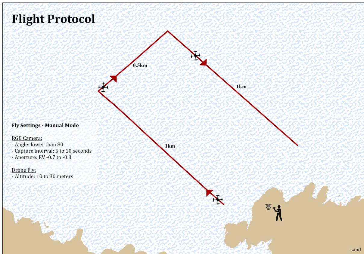
**Figure 2:** Summary of basic flight operations for land-based transect survey for monitoring floating litter contamination (transect distance and values used on Mavic 2 Pro quadcopter; adapt depending on drone model, sensor size, camera and range).
