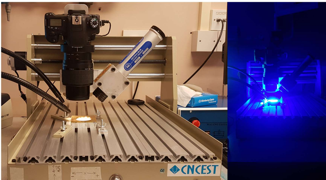
Figure A2.1 Experimental set-up of the digital imaging acquisition system using white light and blue light (420-470 nm)
