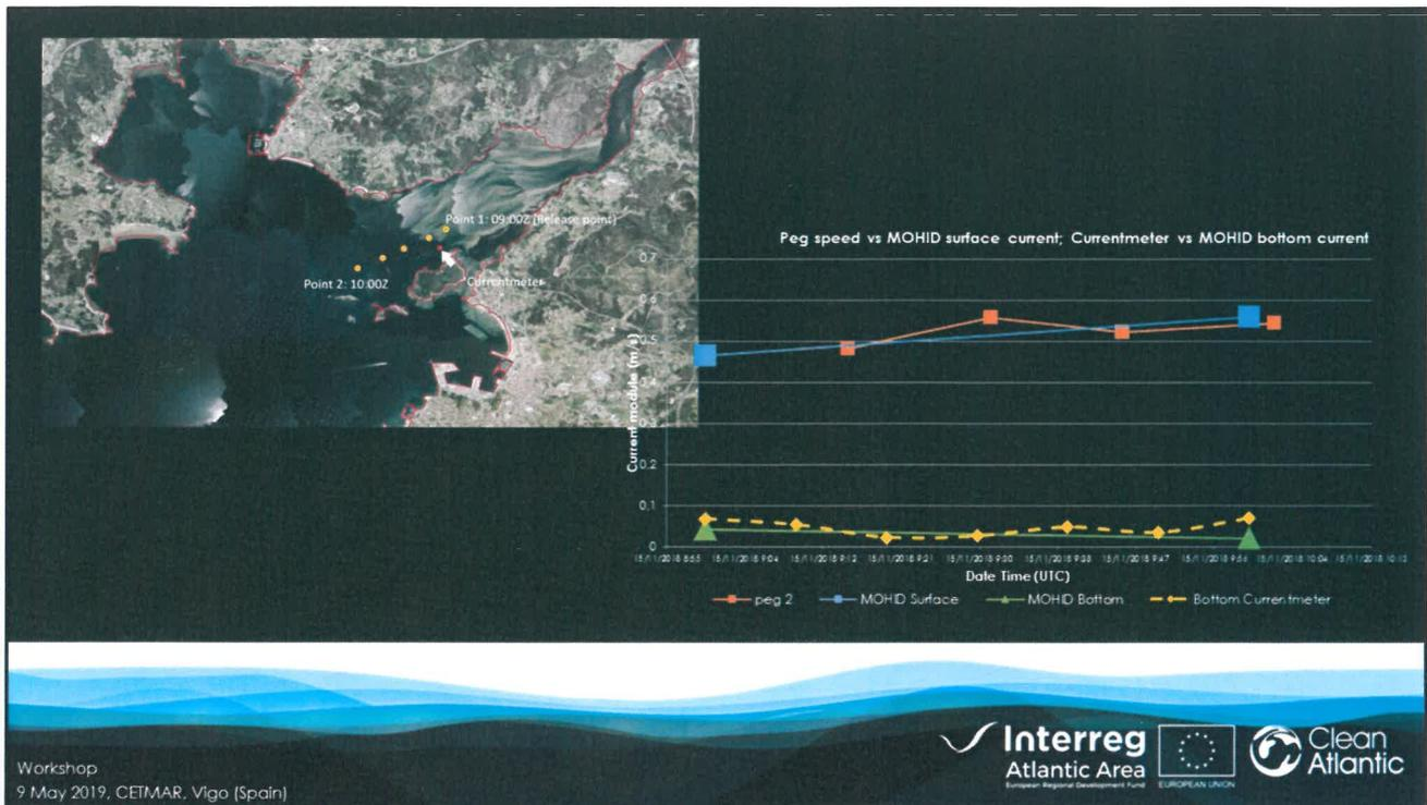
For examples, some pegs were released and the velocity of pegs and surface current forecasted by the model nicely agree. At the same time the model bottom current matches with a measured current.
