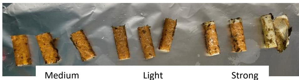
Figure 30: The three types of CB after 9 months of ageing in the Cedre's basin.
