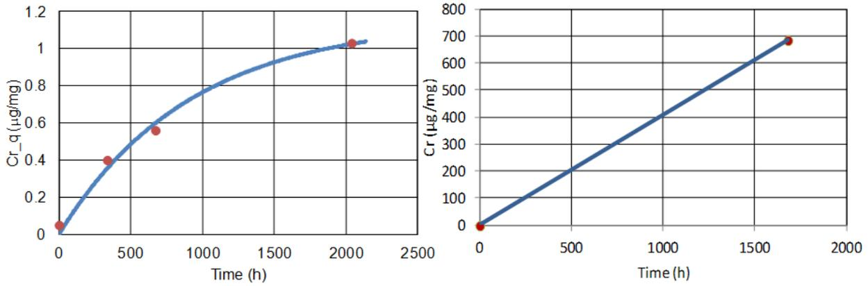
Figure 36: Chromium concentration in medium-strength CBs with time once placed in the sandy beach (left) or in the harbour (right).
